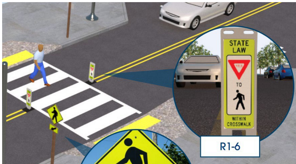
In-Street Pedestrian Crossing Signs (R1-6) (FHWA)
