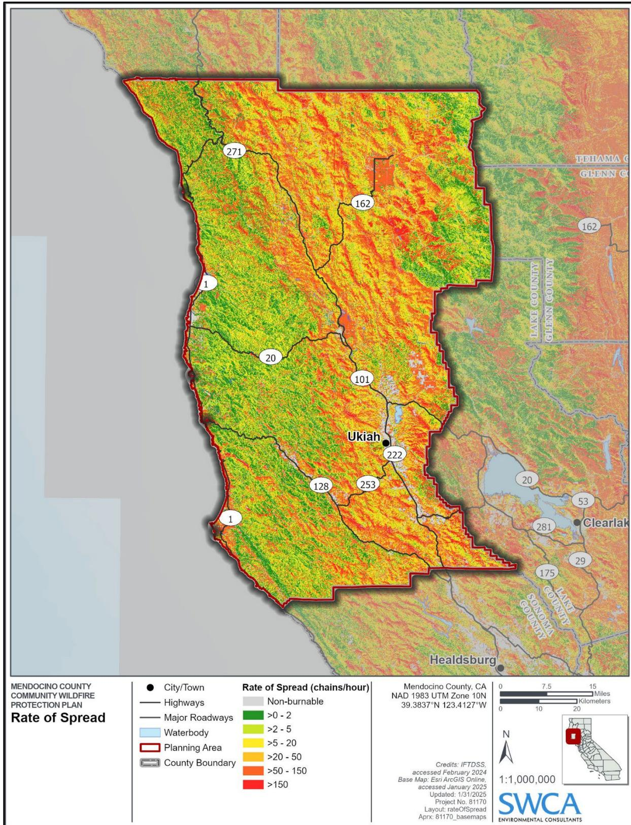
**Figure 3.10. Rate of spread classifications for Mendocino County.** Note: one chain is 66 feet and is a common measure in wildland firefighting. A spread rate of 80 chains per hour is 1 mile per hour.
