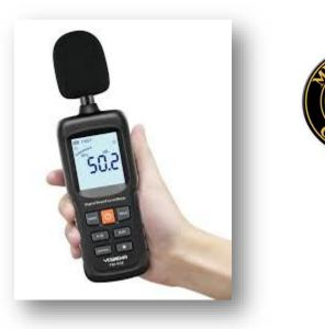
Decibel meters are portable devices to quickly measure sound. Class 1 meters are used, costing \$150 to \$800.
