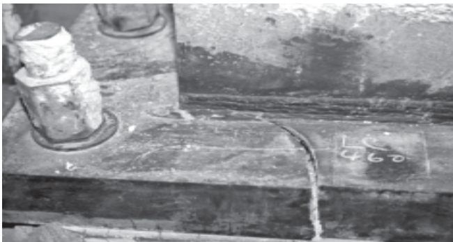
Figure 28 —A 4-inch-thick steel plate supporting the base of a column at the Oviatt Library at CSU Northridge fractured in the 1994 earthquake.
