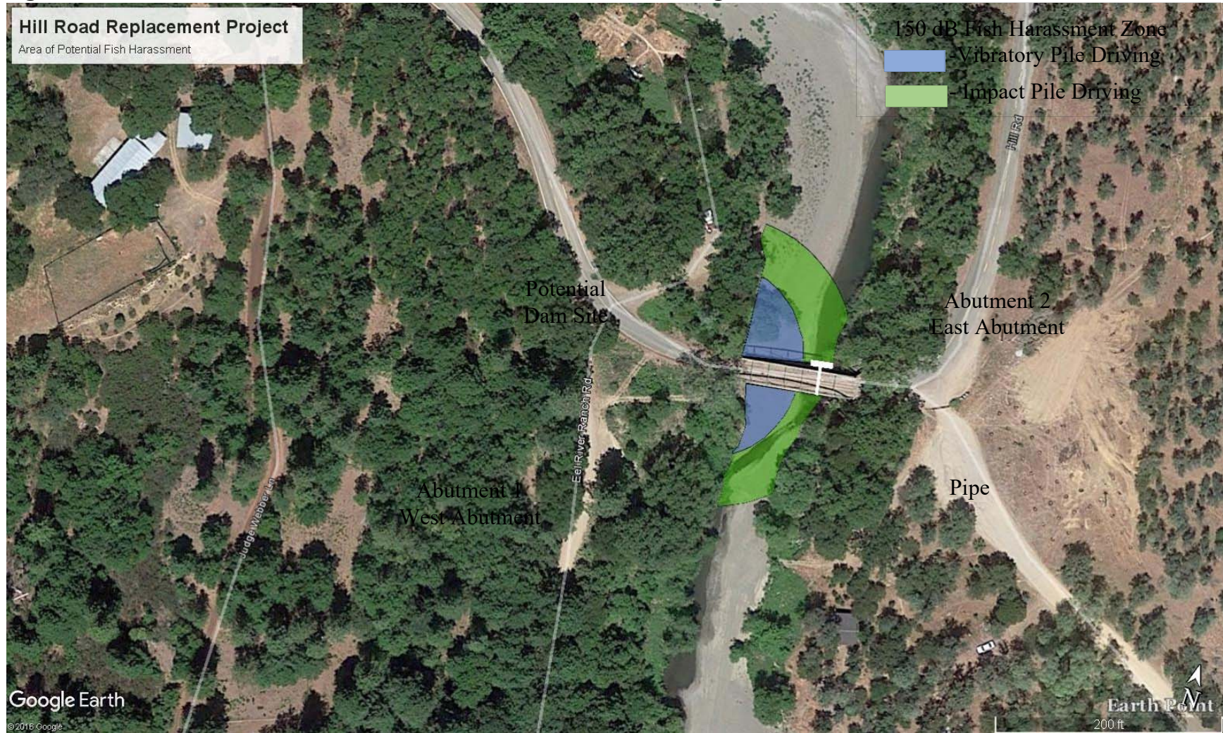
Figure 2 - Hill Road 150 dB RMS Fish Harassment Zone from Pile Driving.
