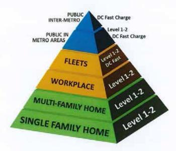
**Level 1** charging can be done through a standard 120V outlet. Level 1 charging is the option used by many people for home charging with a gain of approximately 4 miles of range per hour of charging.
